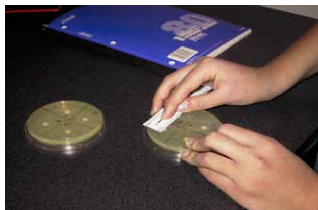
Figure 6. A ruler can be used to measure the zone of inhibition around a compound impregnated disc and student can collect quantitative data and perform statistical analysis.
