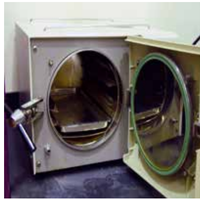
Figure 1. Left: A large industrial size autoclave; cost $10,000+ plus plumbing and electrical work required. Middle: A small table-top autoclave; cost ~$2000 - $5000 or more. Right: A household microwave; cost $100 or less.
