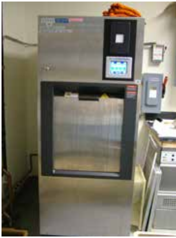
Figure 1. Left: A large industrial size autoclave; cost $10,000+ plus plumbing and electrical work required. Middle: A small table-top autoclave; cost ~$2000 - $5000 or more. Right: A household microwave; cost $100 or less.
