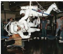
Two astronauts practice space rescue over the Precision Air Bearing Platform (PABP) at the NASA Johnson Space Center. (The PABP is like a giant air hockey table.)
