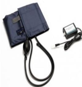
Figure 1: Vernier blood pressure sensor cuffs (BPS-BTA)
