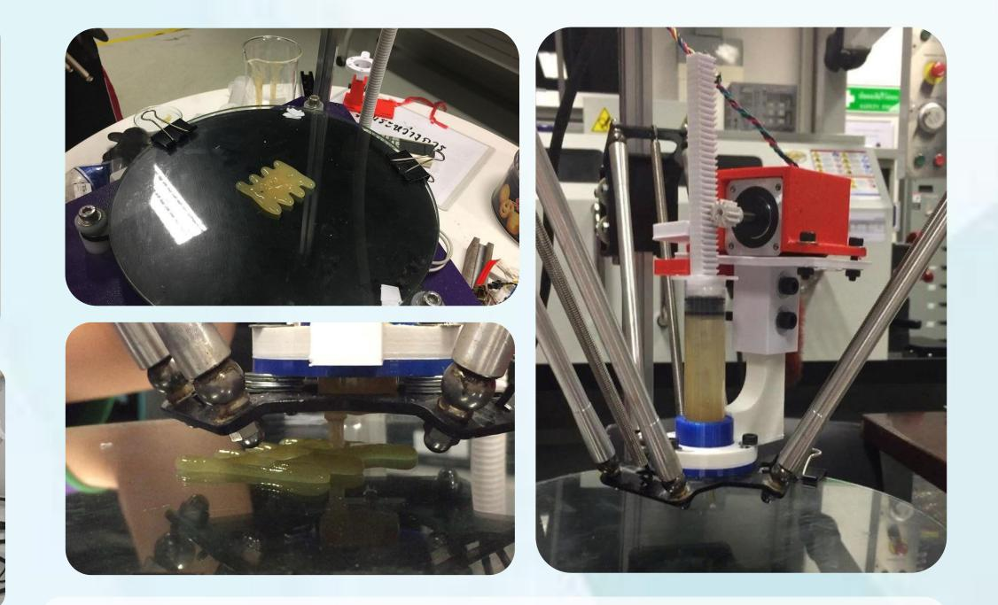
A 3D-printer need to be modified to suitable for gel printing. It has been designed and modified at the first stage in the picture above to test its work. It will be modified and added up until completed to be able to do sol to gel printing method.
