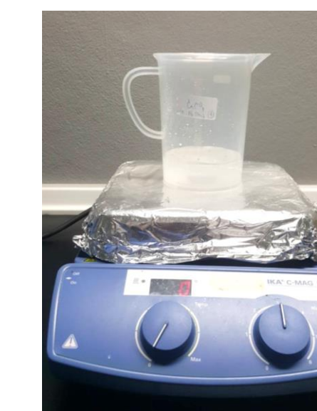
Figure 6. Batch experiment for determining Pb 2+ adsorption capacity of eggshells.
