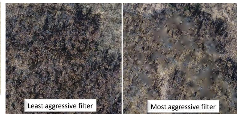
Figure 4. Least aggressive filtering orthomosaic has visibly less blurriness.
